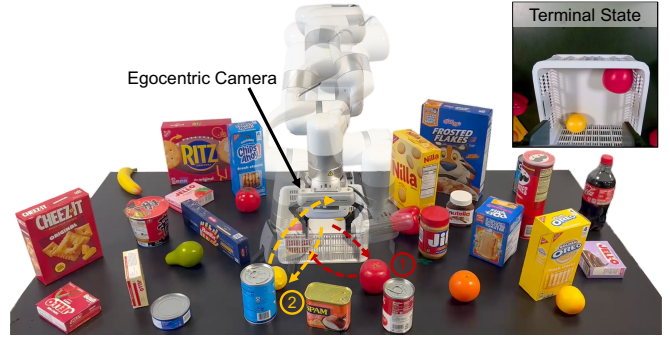
Fig. 8: Real-world setup mirroring the sequential manipulation task from simulation. Our policy is transferred from simulation to the real robot in a zero-shot manner and completes the task.
